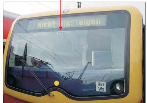
Very small Optical Receiver behind the windshield
